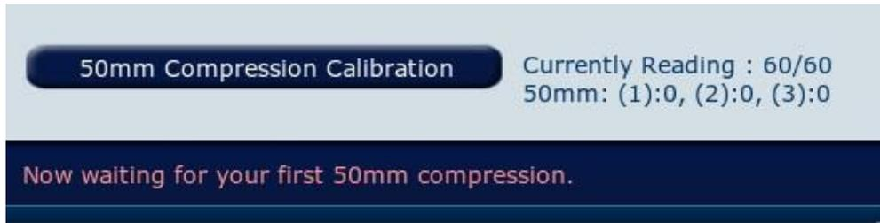
Now press the chest until the pointer (see the green circle in the picture above) moves to 50mm. Speed is NOT important here. Press slowly until the marker is exactly on the 50mm marker. You must do this 3 times as precisely as you can.
